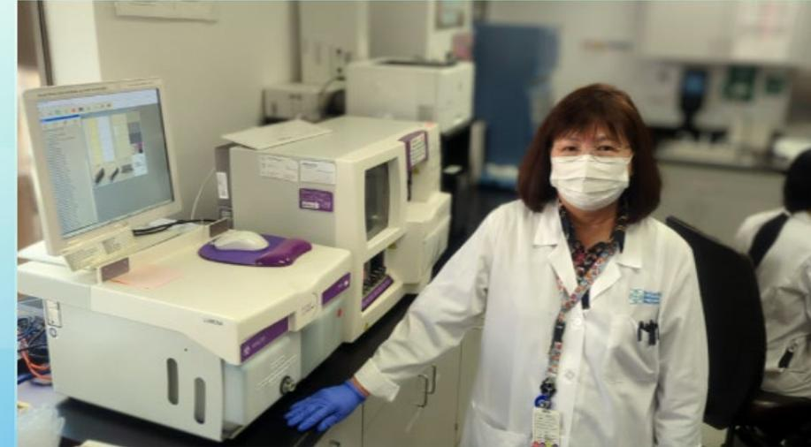
New Echo Lumena Automated Analyzer for Blood Types, Antibody Screens, Donor Unit typing, and Antibody Identification.
